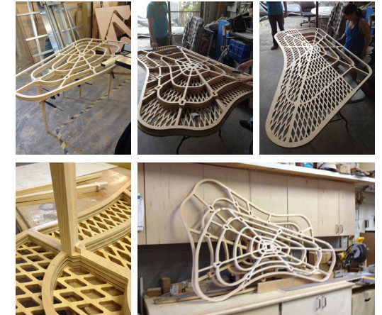
FABRICATION Individual frames were fabricated to accept legs which plug in to custom sockets. Frames were steamed and glued and thin wooden tops were attached to the frames to act as a structural skin. Seen at bottom left is the detail of an individual leg plugged into the organically shaped frame below the thin table top.
