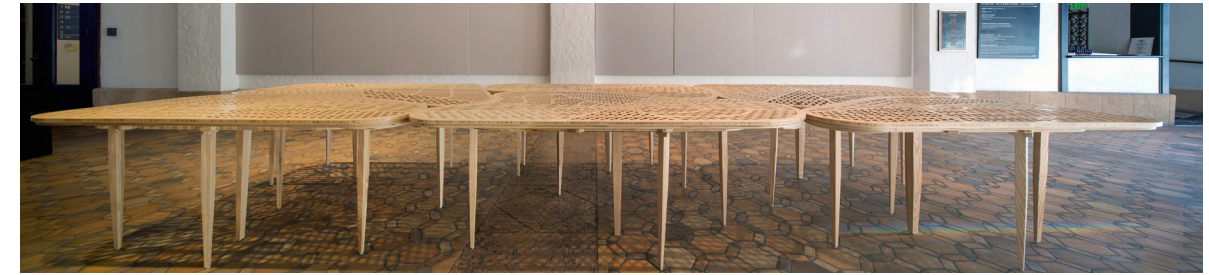
ELEVATION Long side elevation of all table fit snugly together. Due to the non-repeating structural grid below, the structure needed to be selectively thickened to provide stability once all tables were assembled side by side.
